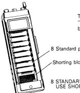
The 75-790 requires 8 penlight "AA" batteries and shorting block for normal operation.
