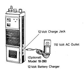
WARNING: Do not attempt to recharge standard penlight carbon cells or alkaline batteries. Recharging must only be done with nickel cadmium rechargable batteries which are labeled rechargable.
